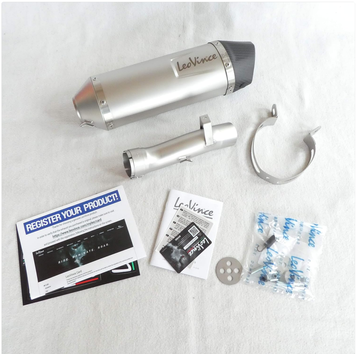
Figure 1: Complete Leovince LV ONE EVO SLIP-ON exhaust system kit.
