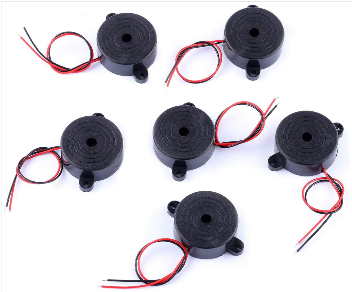
Figure 3.1: Overview of the six Cylewet CYT1117 electronic buzzers included in the package. Each buzzer features a black plastic housing and red and black power wires.
