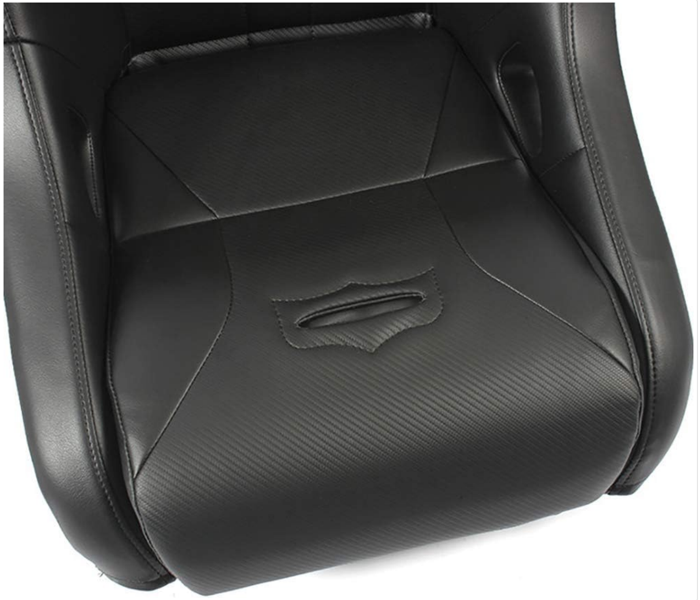
Figure 5.1: Close-up of the seat base, showing the integrated sand drain feature.
