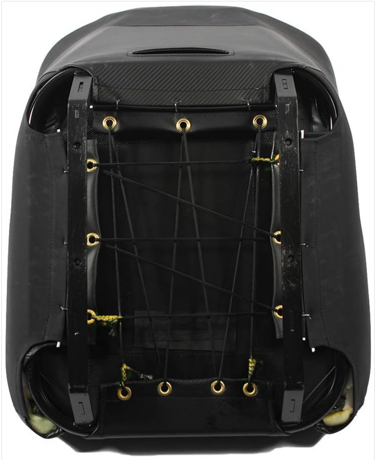
Figure 4.4: Underside view of the Pro Armor G2 Seat, showing the robust frame and suspension webbing.
