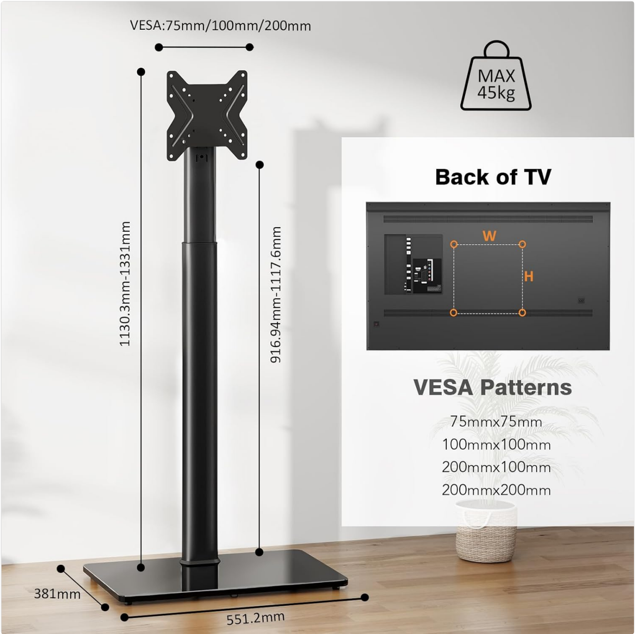
Image 3.1: This image illustrates the dimensions of the stand and various VESA mounting patterns (75x75mm, 100x100mm, 200x100mm, 200x200mm) supported by the TV mounting bracket. It also indicates the maximum weight capacity of 45 kg.
