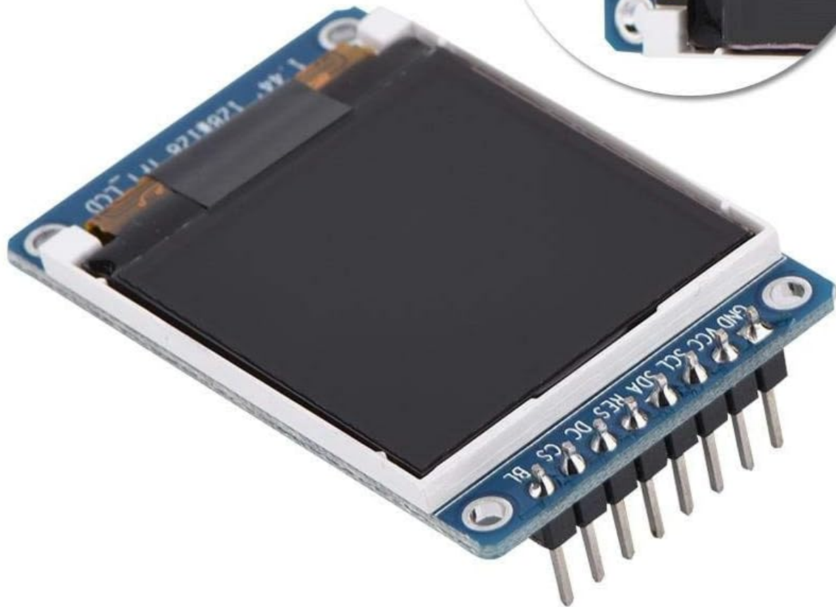
Figure 2.1: The DollaTek 1.44 Inch TFT LCD Module, highlighting its ST7735 controller chip.
