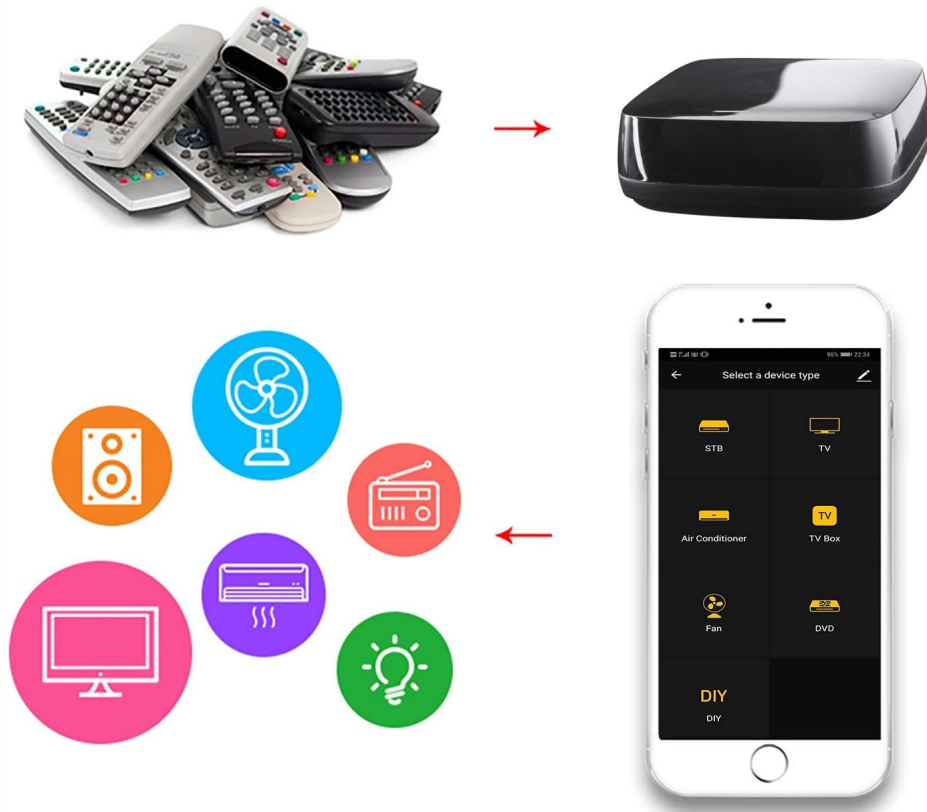
Figure 5.4: Illustrates the DIY learning function, showing how the Woorx remote can learn commands from existing infrared remote controls, expanding its compatibility.
