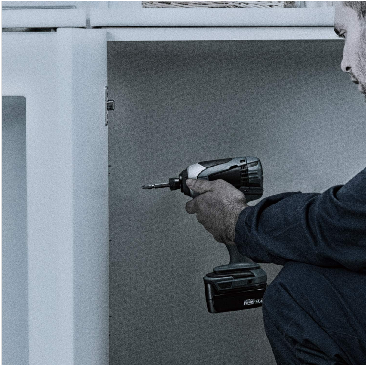
Image 4.2: Example of an impact driver being used with a VESSEL bit for fastening.
