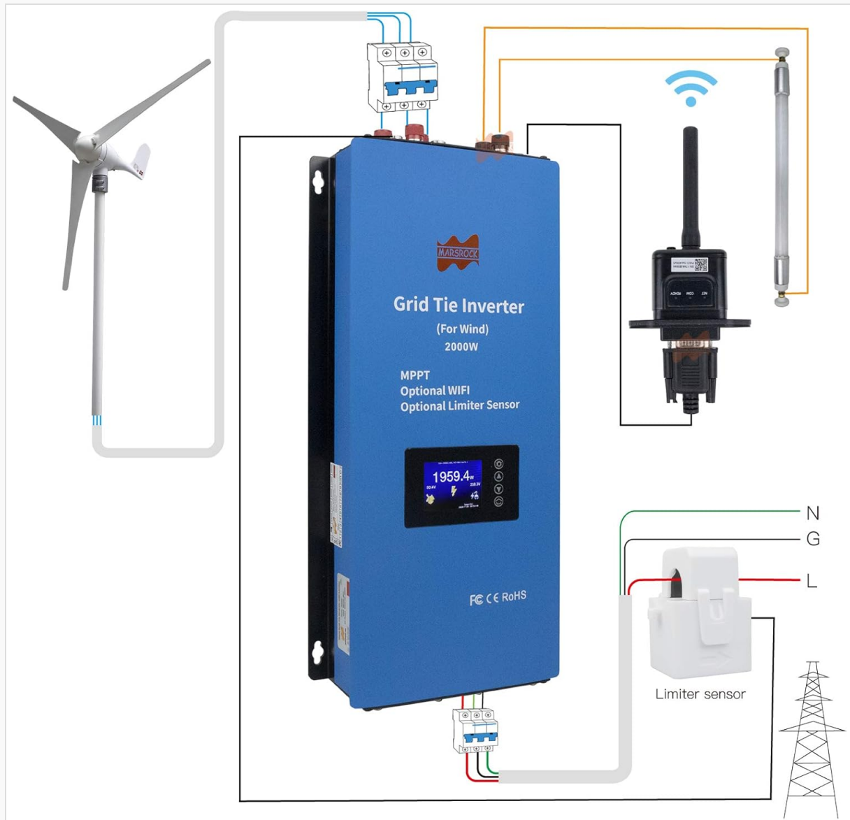
Figure 5: A typical wiring diagram illustrating the connection of the wind turbine, inverter, limiter sensor, and household grid.
