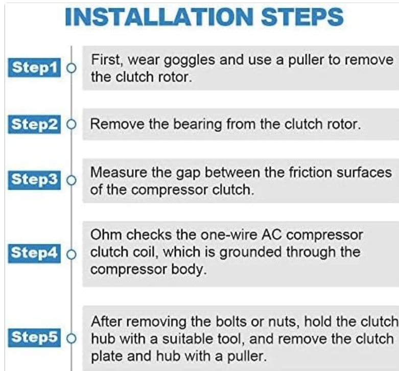
Image: Diagram illustrating the five key steps for A/C clutch installation.
