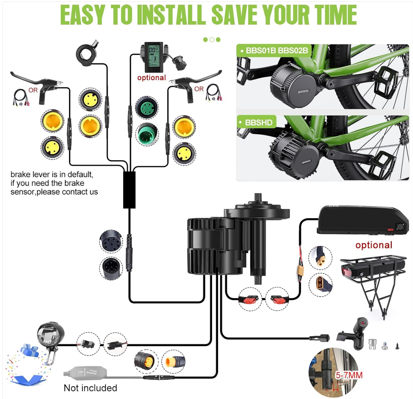
Image: Easy Installation Wiring Diagram. This diagram illustrates the connections for the BAFANG mid-drive motor kit, including the motor, display, brake levers/sensors, throttle, speed sensor, and optional battery and lights. It emphasizes the waterproof wiring.
