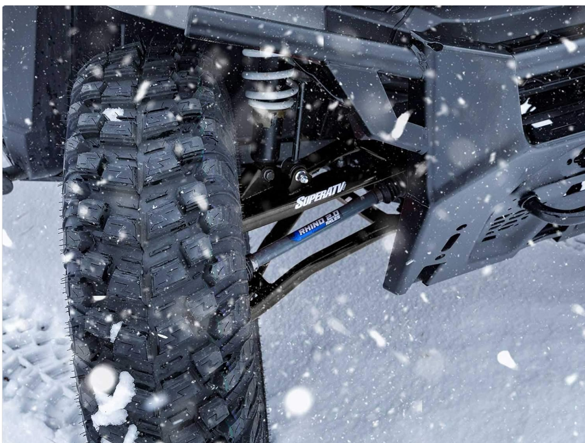
Image 5.3: Front wheel area of a Polaris Ranger with the SuperATV BFT Suspension Kit installed, highlighting the new A-arms and increased clearance.
