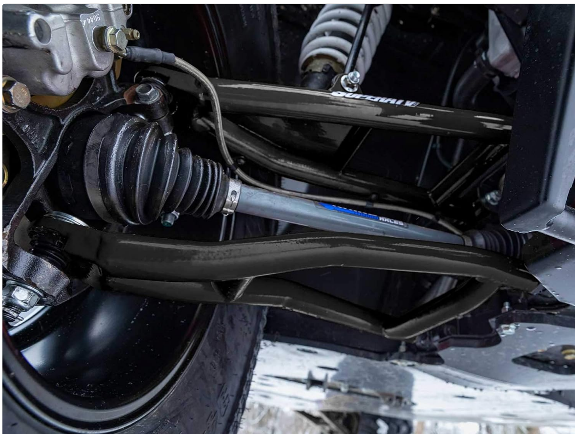
Image 5.2: Another view of the installed A-arms, showing their robust construction and clearance around the axle.
