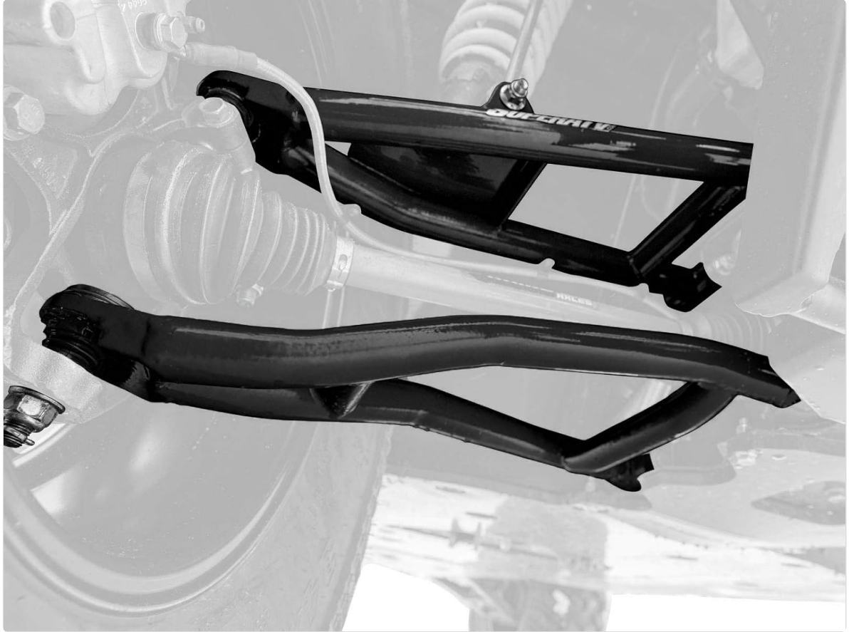
Image 5.1: Close-up of the SuperATV BFT A-arms installed on a vehicle's front suspension.
