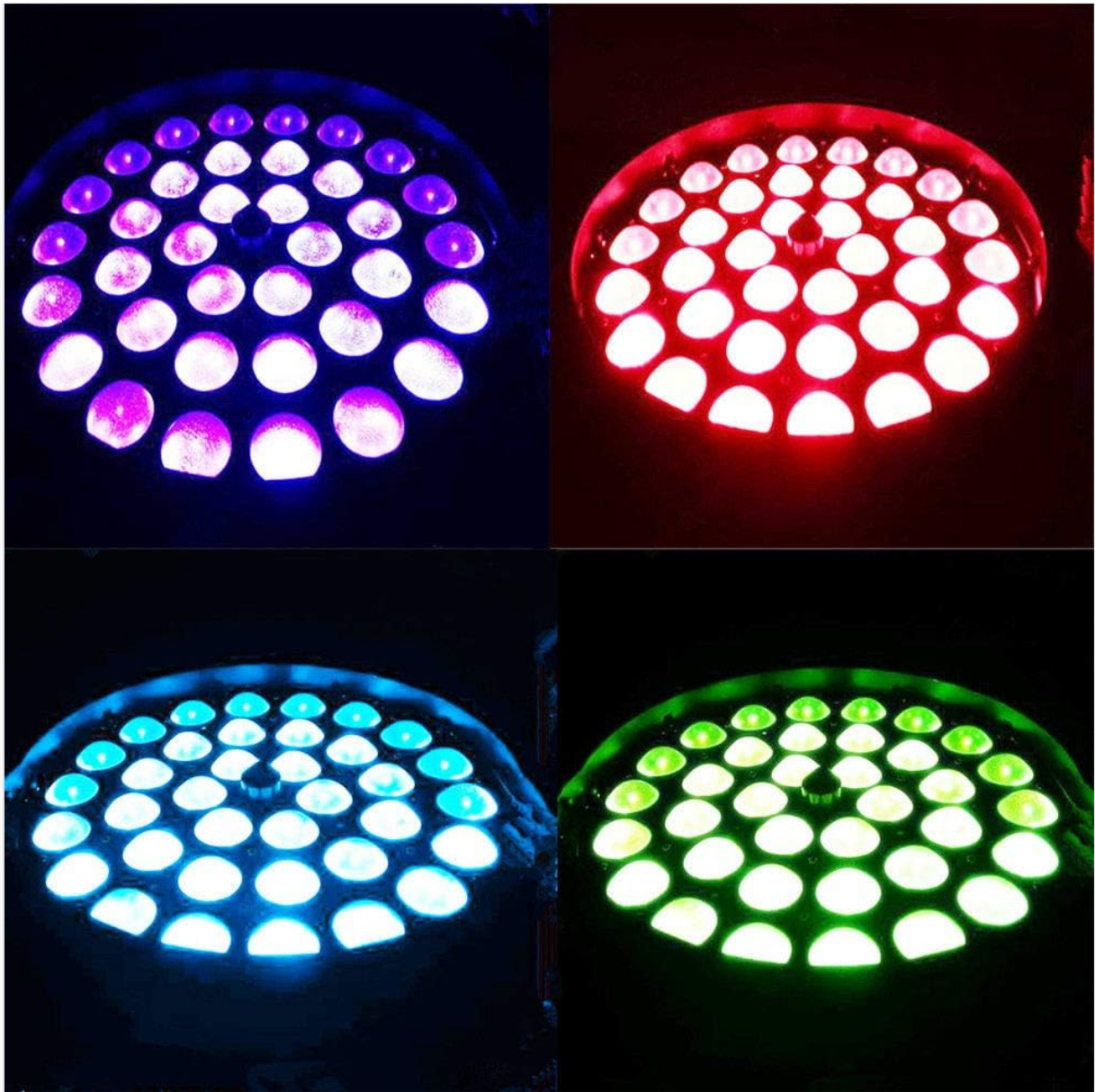
Figure 4: A detailed view of the LED array, demonstrating the individual RGBW LEDs illuminated in different color combinations, showcasing the ring control capability.
