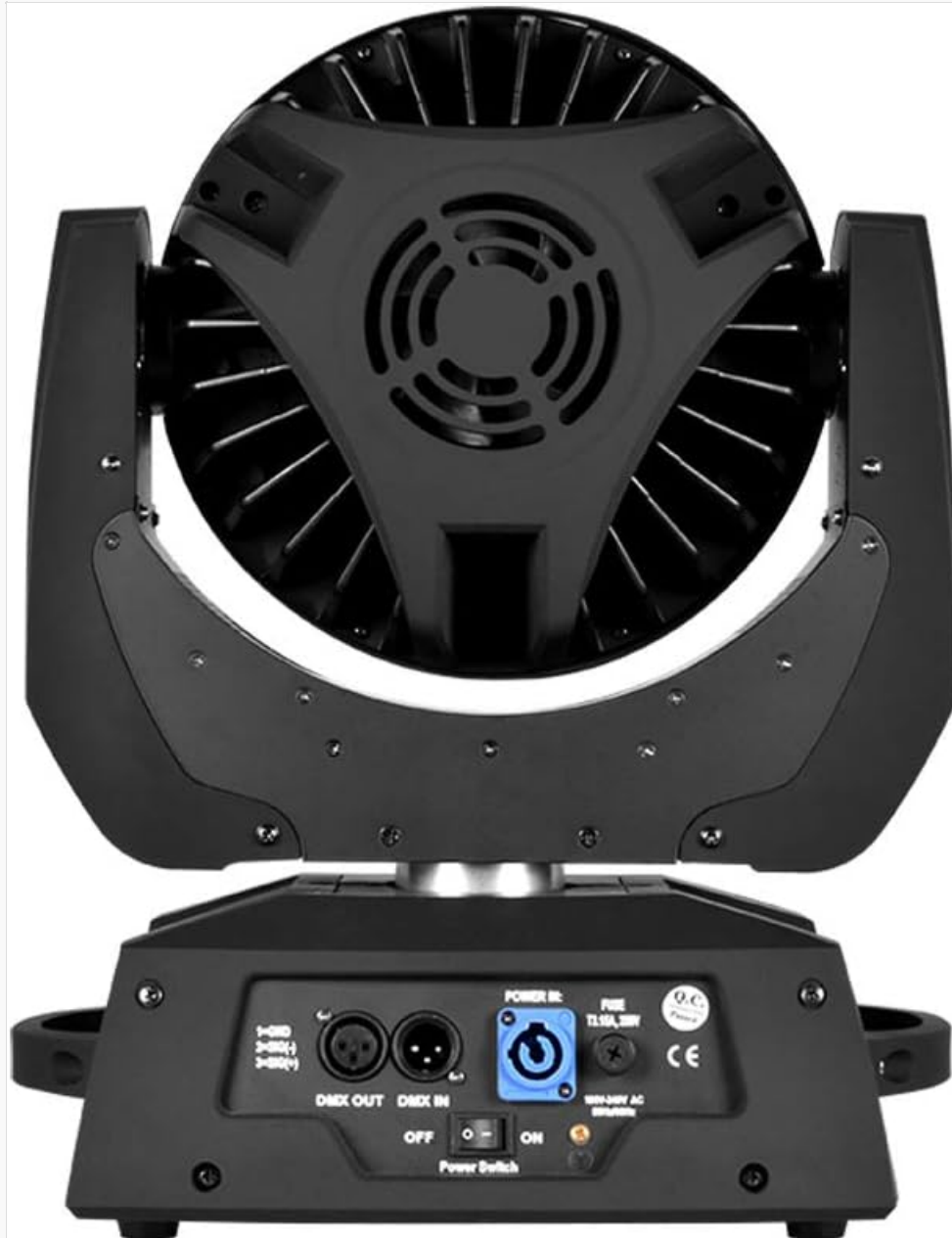
Figure 2: The rear panel of the stage light, highlighting the Powercon IN/OUT and 3-pin DMX IN/OUT connectors, along with the power switch and fuse.
