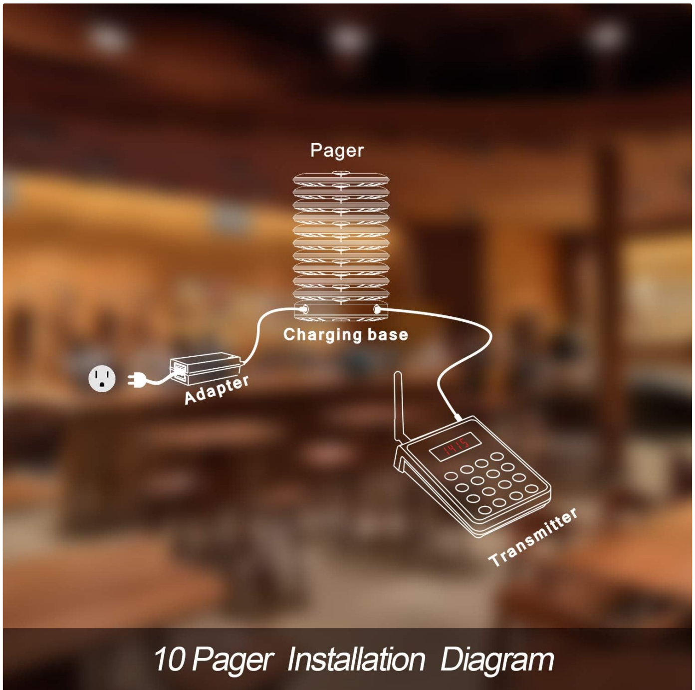
Image 4.1: Installation diagram illustrating how the transmitter, charging base, and adapter connect with the pagers.
