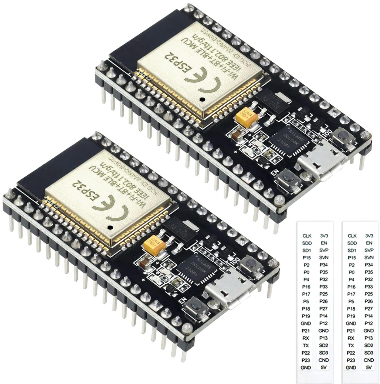
Figure 1: Two KeeYees ESP32S 38-PIN development boards. These boards offer integrated Wi-Fi and Bluetooth for various development projects.
