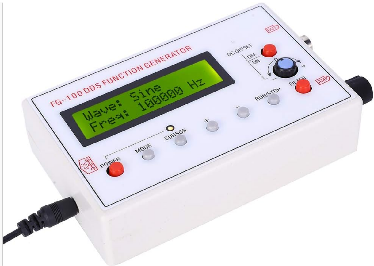
Figure 4.1: The FG-100 generator with the DC power cable connected to the input port.
