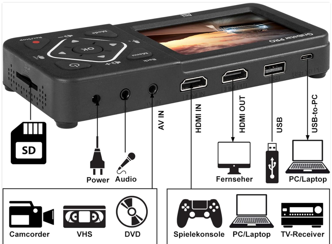
Image: A comprehensive diagram illustrating the various ports on the Grabstar PRO, including SD card slot, power, audio, AV IN, HDMI IN, HDMI OUT, USB, and USB-to-PC, along with examples of devices that can be connected to each port (Camcorder, VHS, DVD, Gaming Console, PC/Laptop, TV-Receiver).
