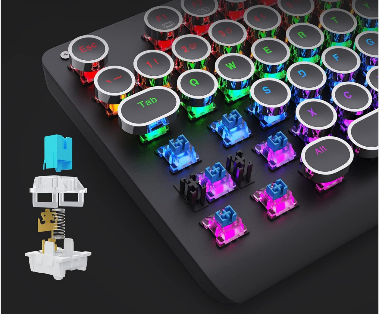
Figure 4: Detail of the mechanical blue switches.
