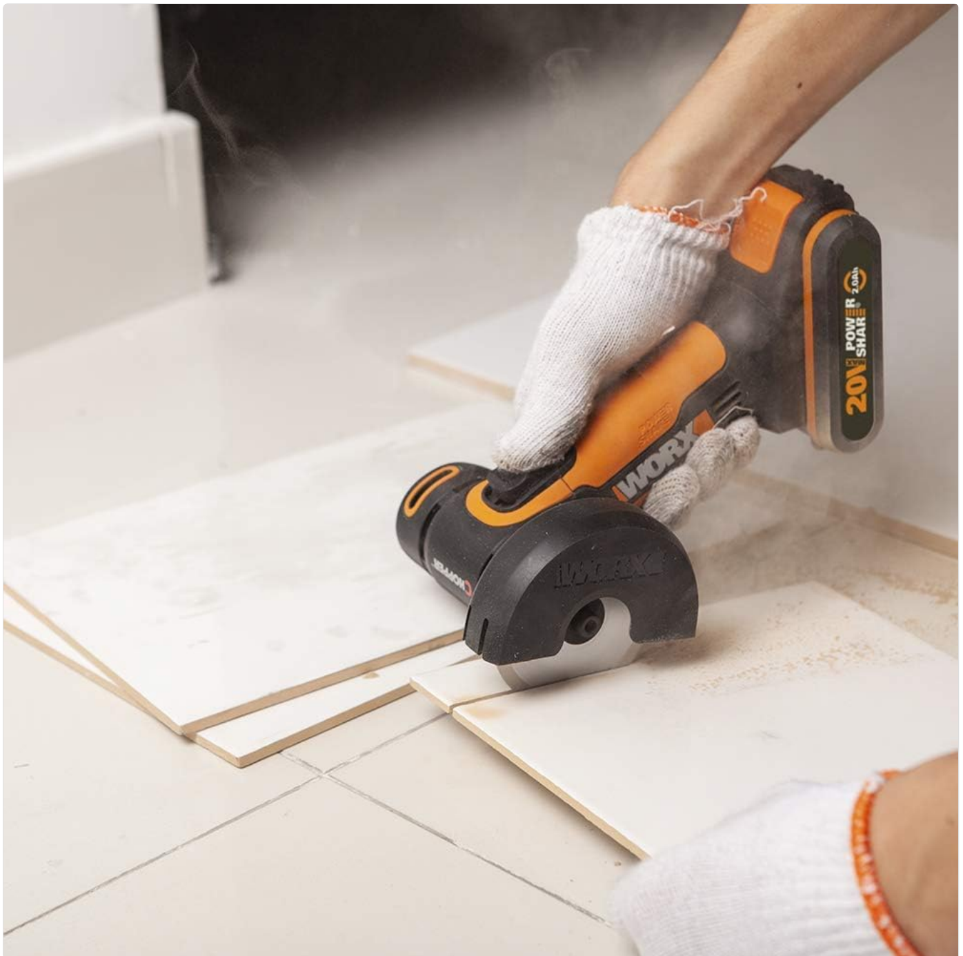
Figure 3: The WORX WX801.9 Mini Chopper Grinder in use, demonstrating its capability to cut through materials like ceramic tiles with precision.
