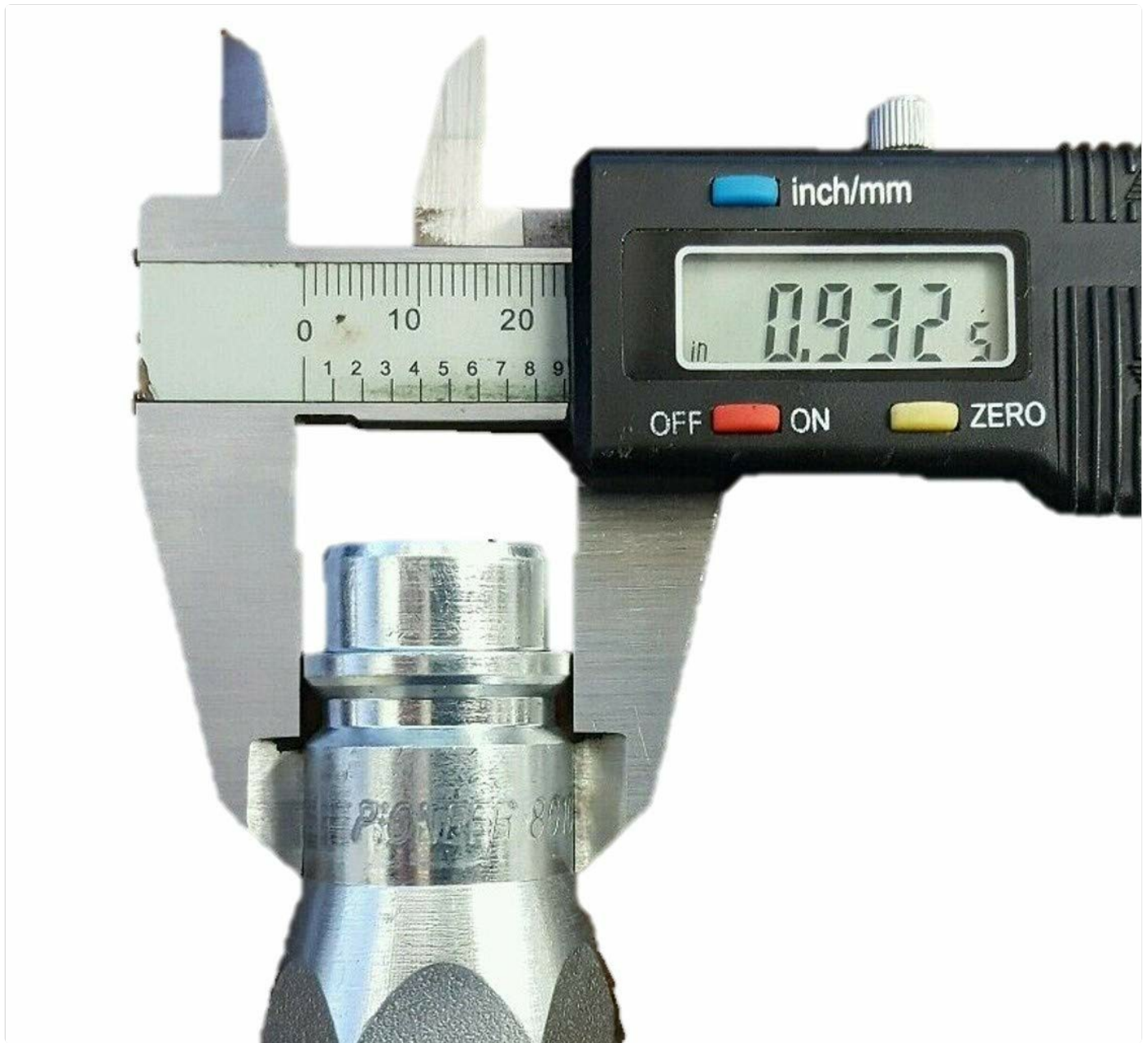
Image 4: Hydraulic Fitting Measurement. This image illustrates the precision required for hydraulic components, showing a digital caliper measuring a fitting, which is crucial for selecting the correct plug or cap size.
