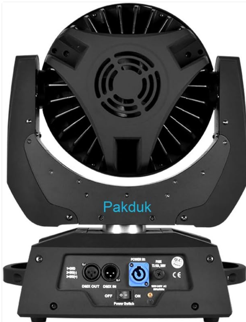
Figure 4.2: Rear view of the Boulder LED Moving Head Wash Light. This view highlights the cooling fan, Powercon IN/OUT connectors, 3-pin DMX IN/OUT connectors, a fuse holder, and the main power switch.
