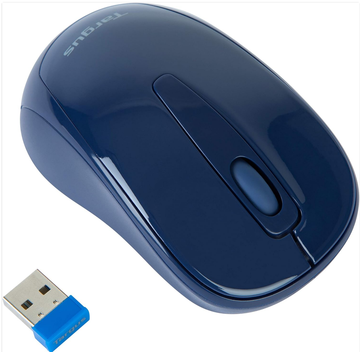
Image: The Targus W600 Wireless Optical Mouse shown with its compact USB receiver, which plugs into your computer's USB port.
