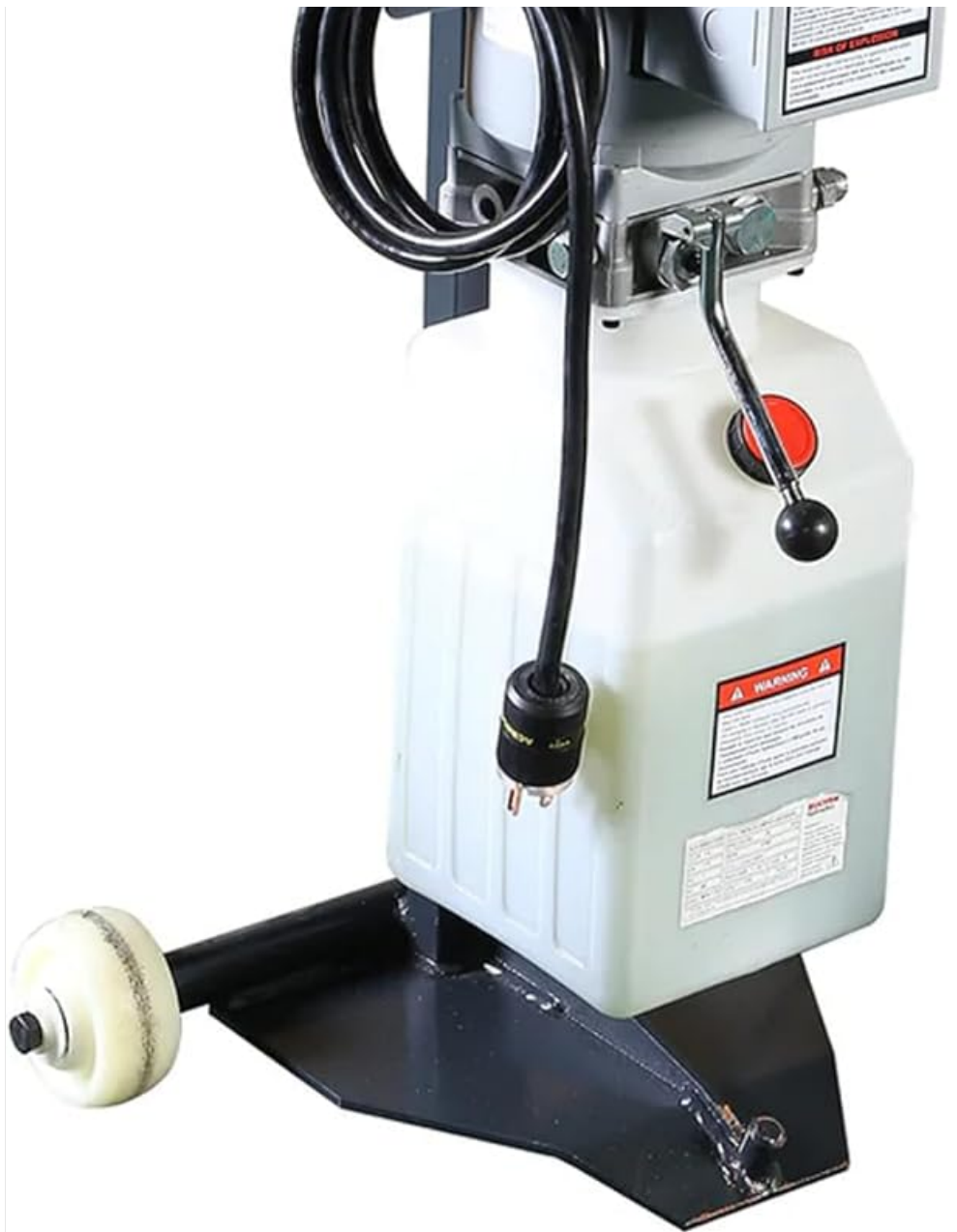
Figure 2.4: The portable 110V power unit, which supplies hydraulic pressure to the lift.
