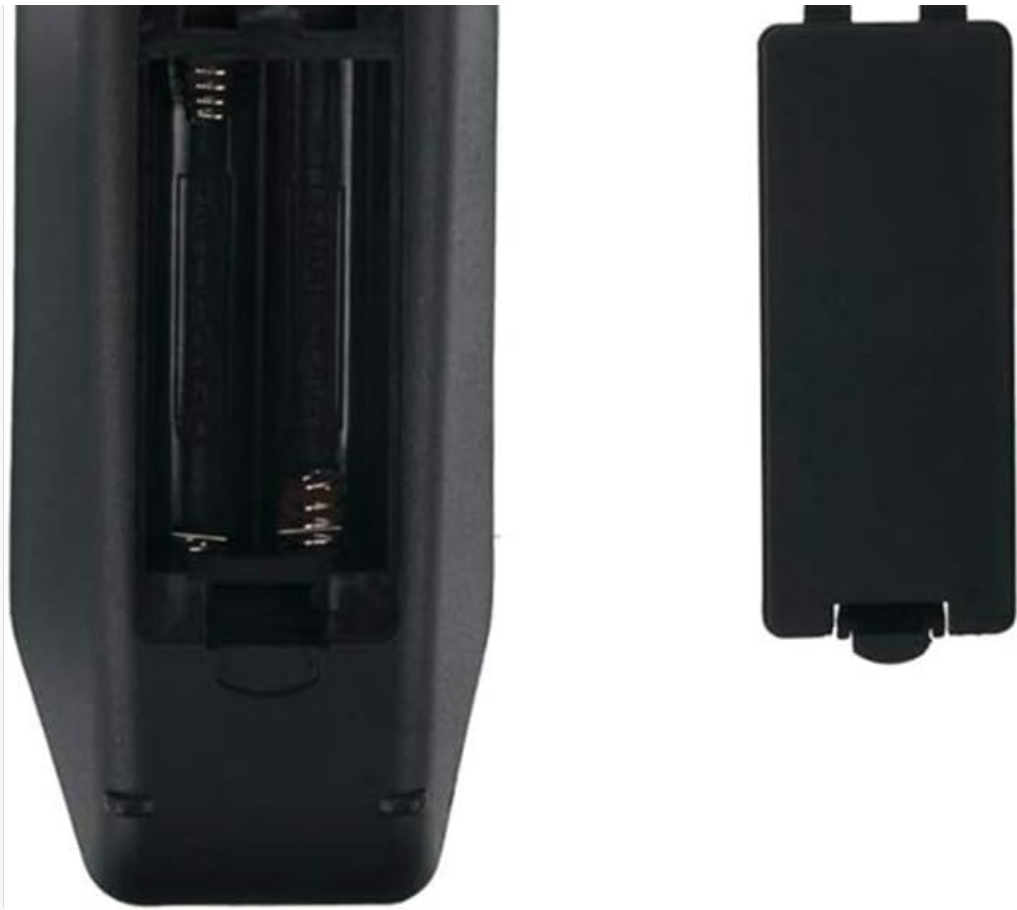
Figure 2: Back view of the remote control with the battery compartment open, showing where to insert AAA batteries.
