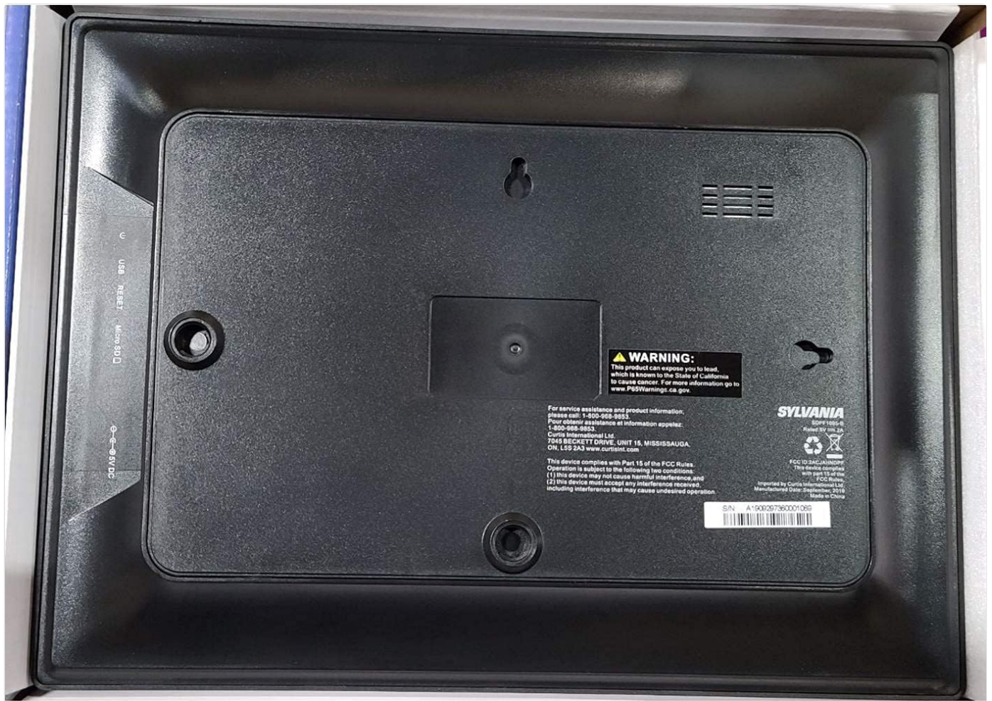
Image: The rear panel of the digital picture frame, illustrating the location of the DC power input, Micro USB port, and MicroSD card slot for connectivity and expansion.
