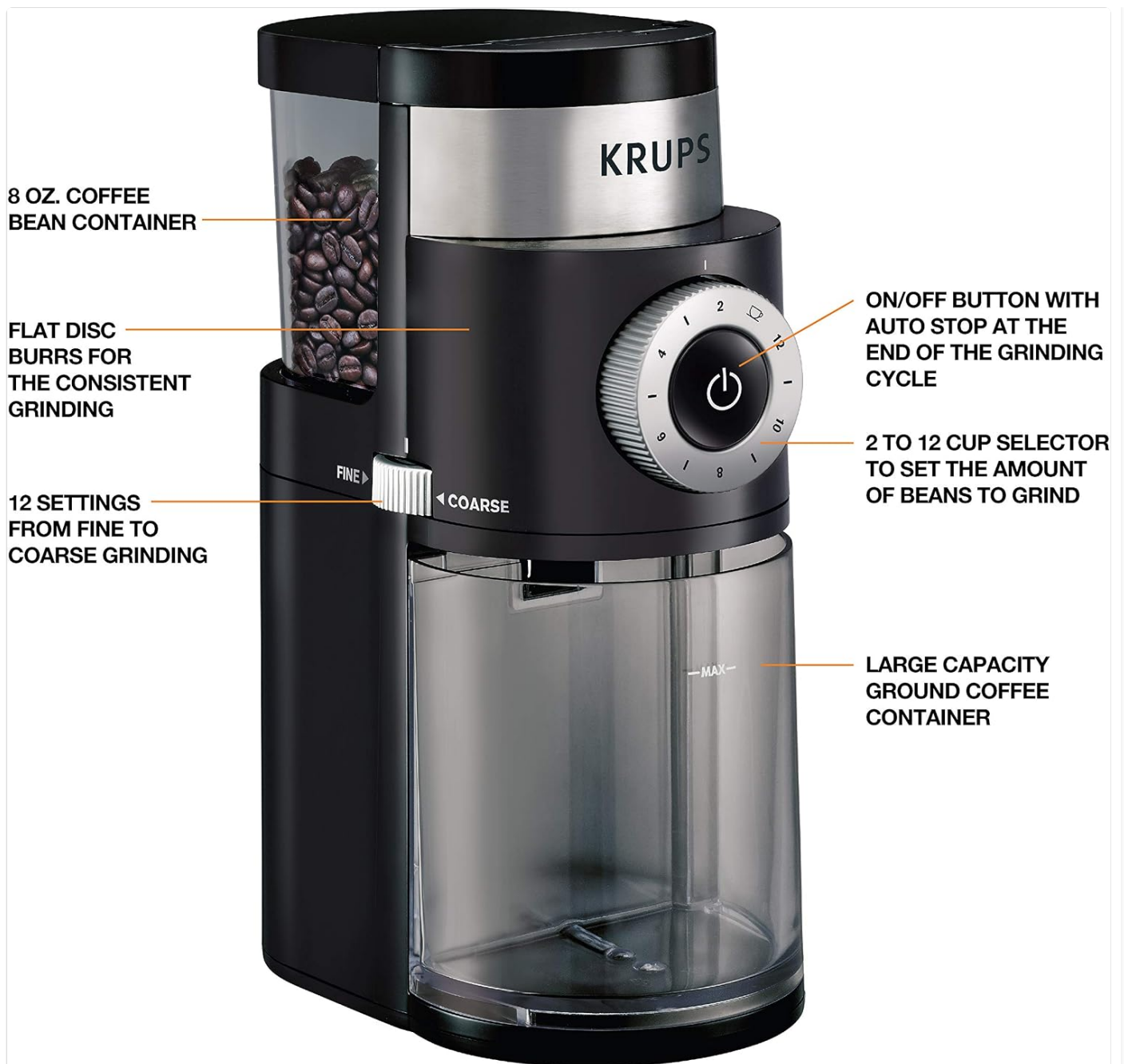
Image 3.1: Labeled components of the KRUPS Precision Burr Coffee Grinder.
