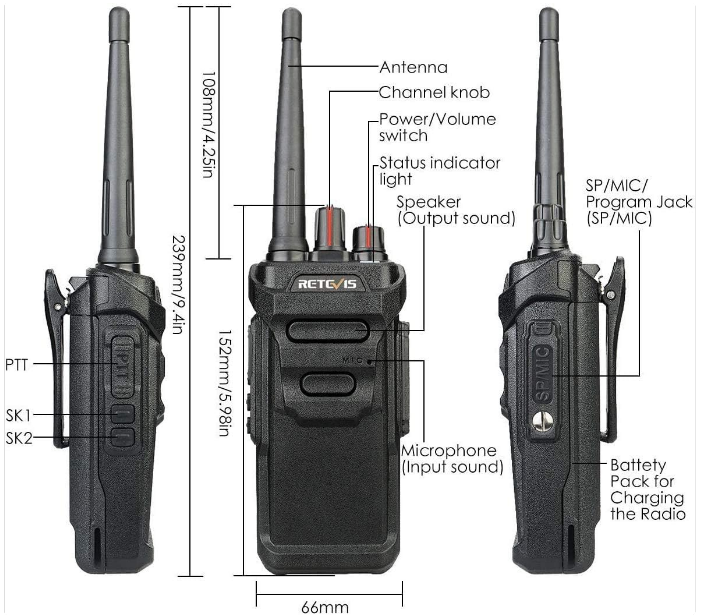
Figure 2.1: Retevis RT648 Walkie-Talkie Components Diagram
