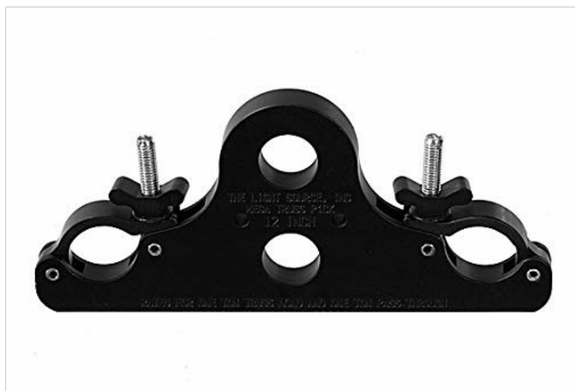
Figure 1: The Light Source MTP12B 12-Inch Mega-Truss Pick. This image displays the main body, the two pockets with coupler-style aluminum pivoting links, and the half-inch swivel bolts with solid wing nuts designed to secure around a truss tube. The top and bottom rigging holes for shackle or motor attachment are also visible.
