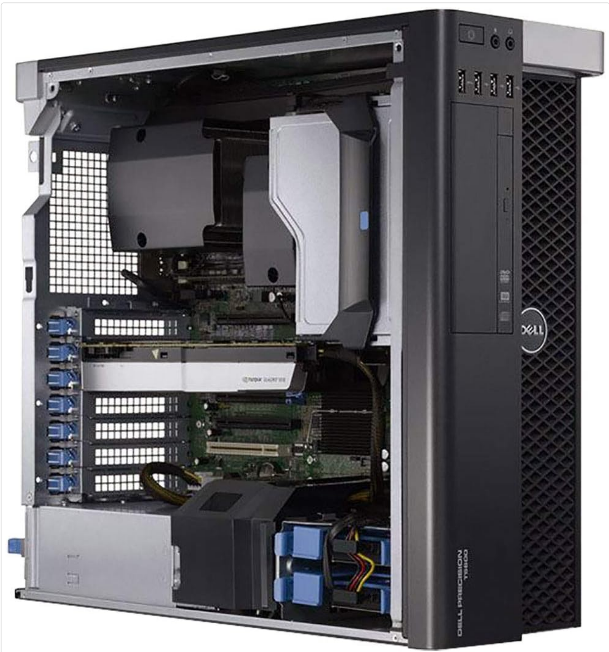
Figure 4: Internal view of the Dell Precision T5610 Workstation, showing the layout of components such as the motherboard, expansion slots, and drive bays. Regular dust removal from these areas is recommended.
