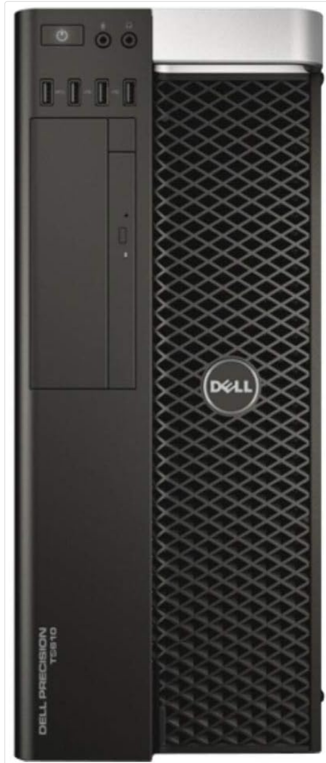
Figure 2: Front view of the Dell Precision T5610 Workstation, showing the power button, optical drive, and front USB ports.
