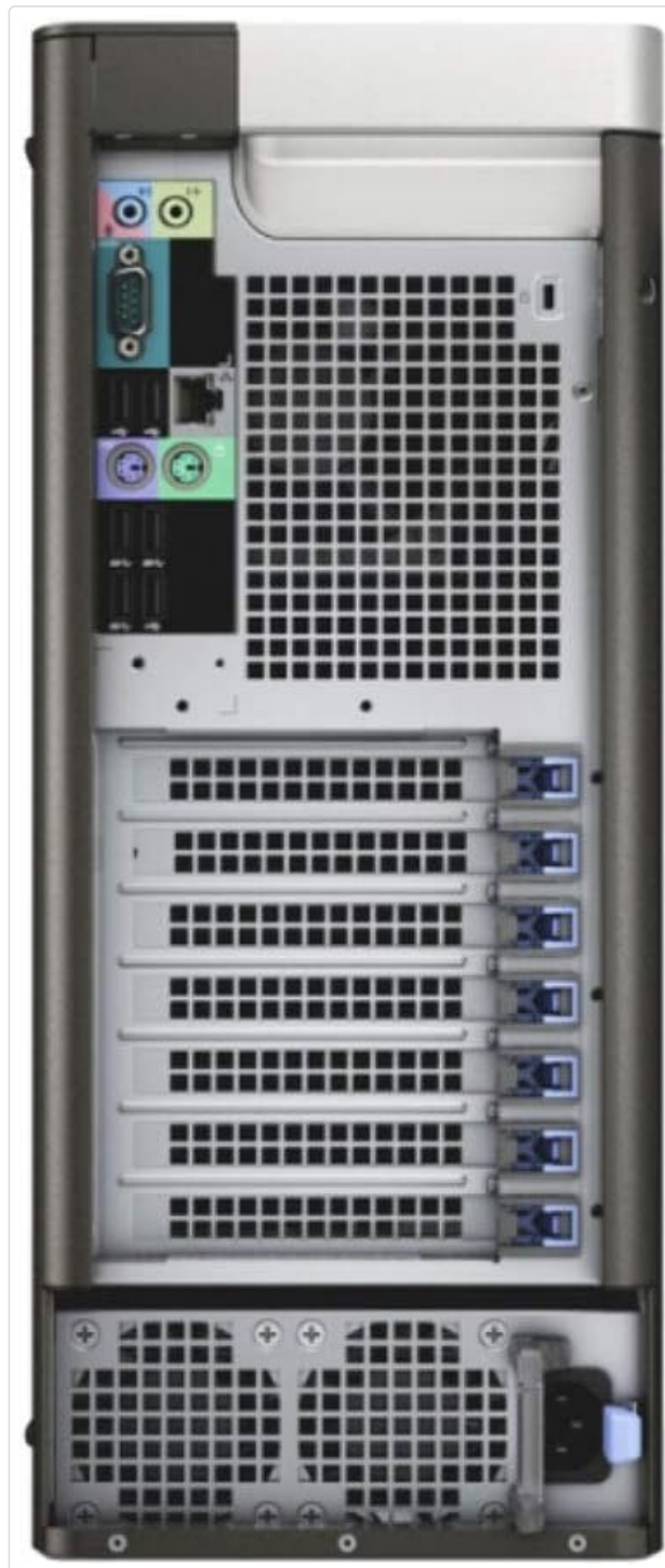
Figure 3: Rear view of the Dell Precision T5610 Workstation, illustrating the various connectivity ports including video outputs, USB, network, and power input.
