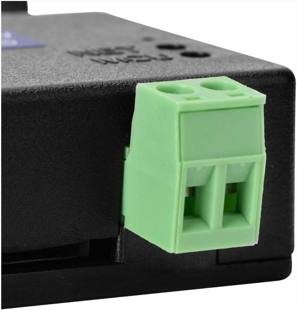
Image: A close-up view of the green terminal block on the GL09 unit, used for power input and connecting external sensors.
