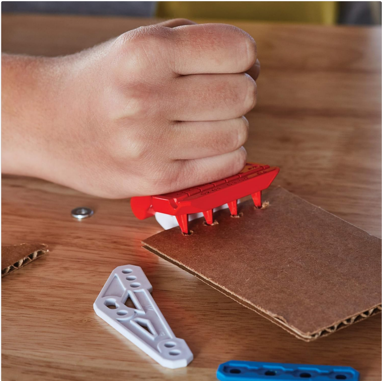
Figure 4.2: The Maker Tool being used to punch holes in a piece of cardboard, illustrating its custom part creation capability.
