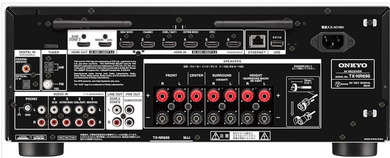
Figure 2: Rear panel of the ONKYO TX-NR696 AV Receiver. This image displays the comprehensive array of input and output terminals, including multiple HDMI ports (supporting 4K/HDCP 2.2), digital audio inputs (coaxial and optical), analog audio inputs, speaker terminals for 7.2 channels, Ethernet port, USB port, and the AC power inlet.
