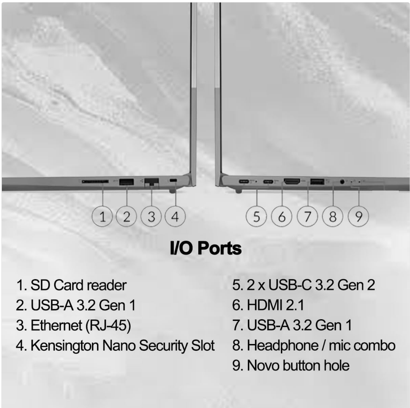
Figure 5: Detailed view of the I/O Ports.
