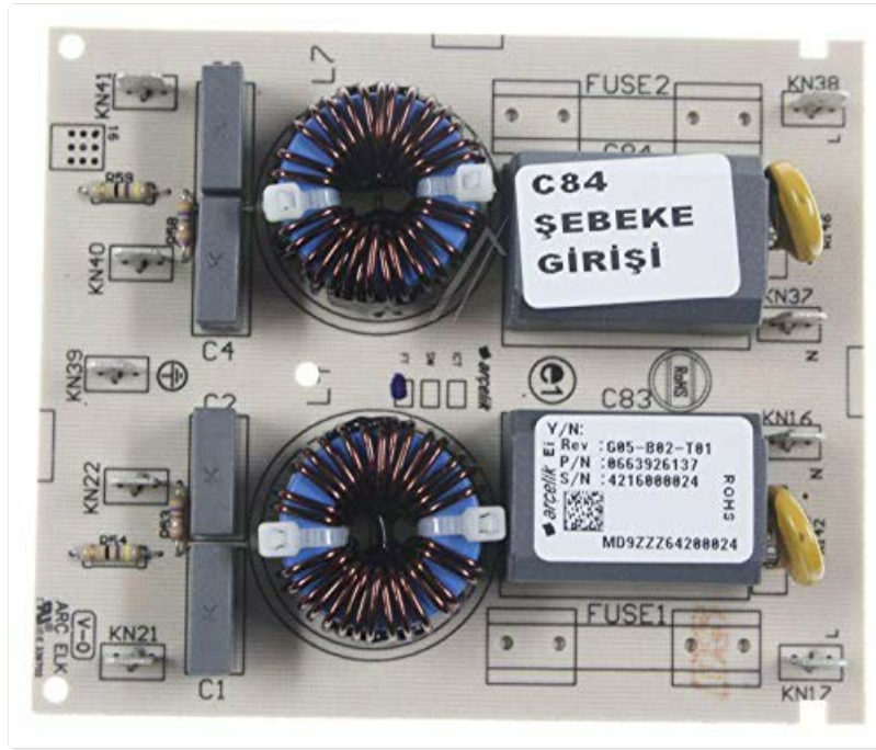
Image of the Beko 663926137 Induction Hob Power Supply Board, showing its electronic components and connectors.
