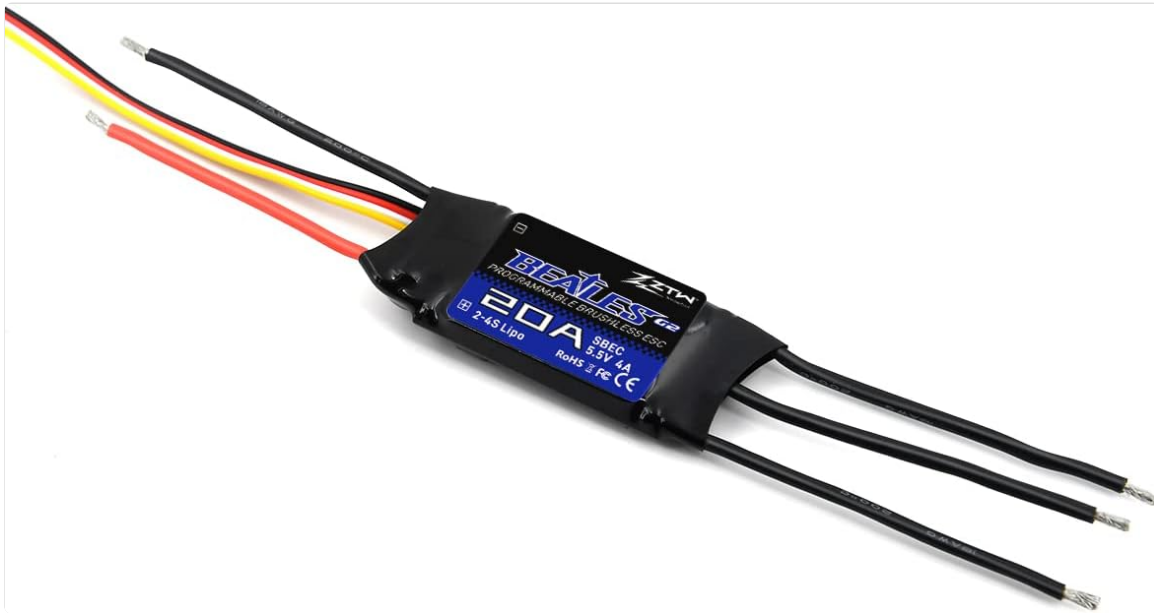
Image: Top view of the ZTW Beatles G2 20A ESC, showing the main body with branding and specifications, and the red/black power input wires on one side, and three black motor output wires on the other.
