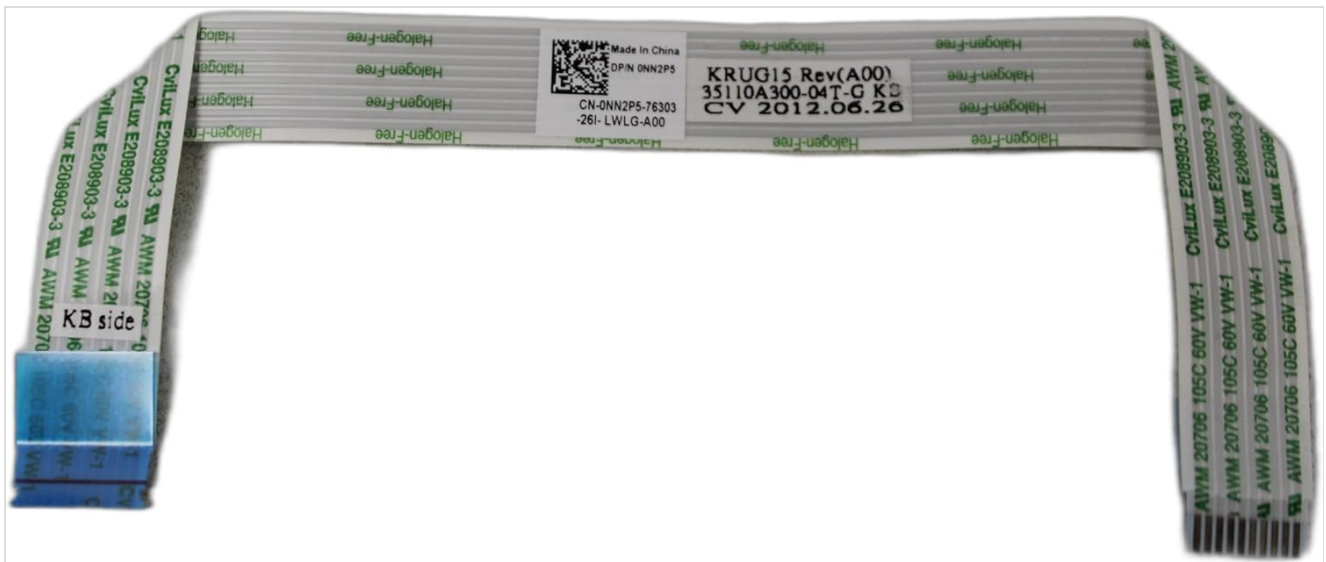
Figure 4.1: Close-up view of the YOTON CN-0NN2P5 Flex Ribbon Wire, highlighting the gold contact pins on both ends. These pins are crucial for establishing the electrical connection within the laptop's ZIF connector.
