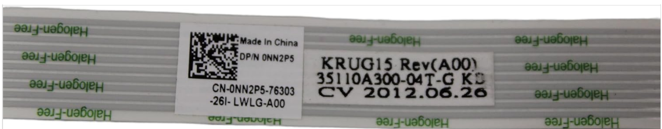
Figure 4.2: Detailed view of the YOTON CN-0NN2P5 Flex Ribbon Wire, showing product markings and specifications printed on the cable. This includes the part number and manufacturing details, which can be useful for verification.
