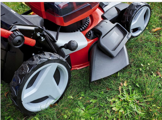
Figure 5.7: View of the mower deck, showing the side discharge and mulching adapter.
