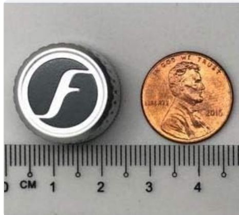
Image: A FOBO Bike 2 sensor is placed next to a US penny and a ruler, illustrating its compact size. The sensor is approximately 2cm in diameter.
