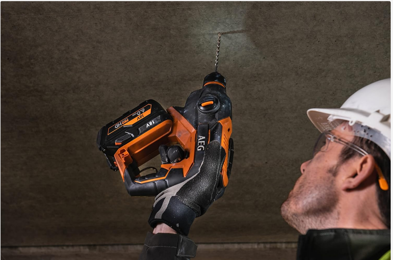
Figure 5: Close-up view of the AEG BBH18C-0 in action, demonstrating its effectiveness for overhead drilling in concrete.
