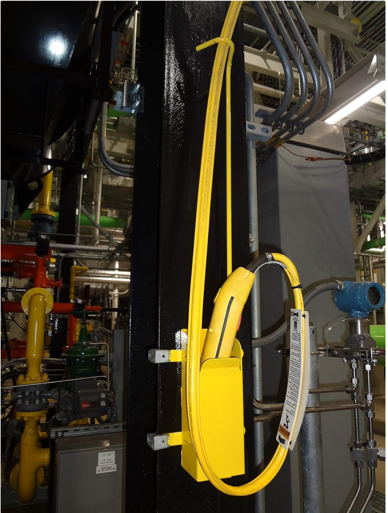
Figure 4.1.1: A crane pendant is shown securely stored in the S-PCM unit, with its cable neatly wrapped around the integrated support arm. This setup ensures the cable is organized and out of the way when not in use.
