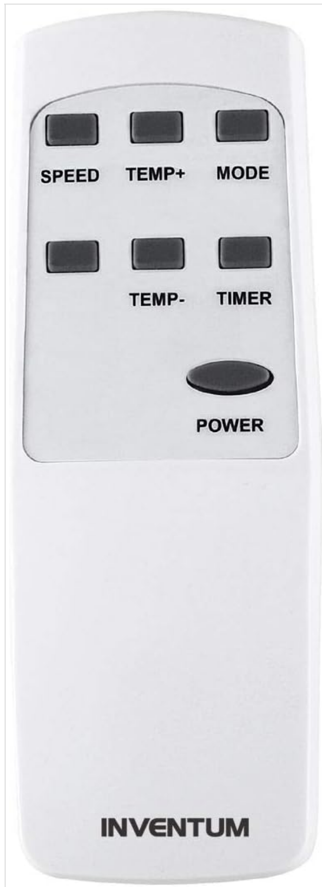
Figure 2.4: The remote control for the AC901, featuring buttons for Speed, Temp+, Mode, Temp-, Timer, and Power, allowing convenient operation from a distance.
