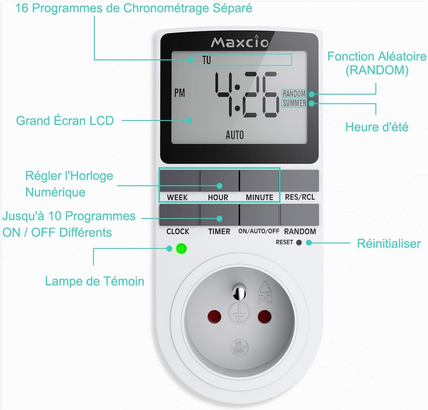
Figure 3: Labeled diagram of the timer plug. This image details the LCD screen, showing the current time, day, and status indicators (PM, RANDOM, SUMMER, AUTO). It also labels the function buttons: WEEK, HOUR, MINUTE, RES/RCL, CLOCK, TIMER, ON/AUTO/OFF, RANDOM, and the RESET button, along with the indicator light.
