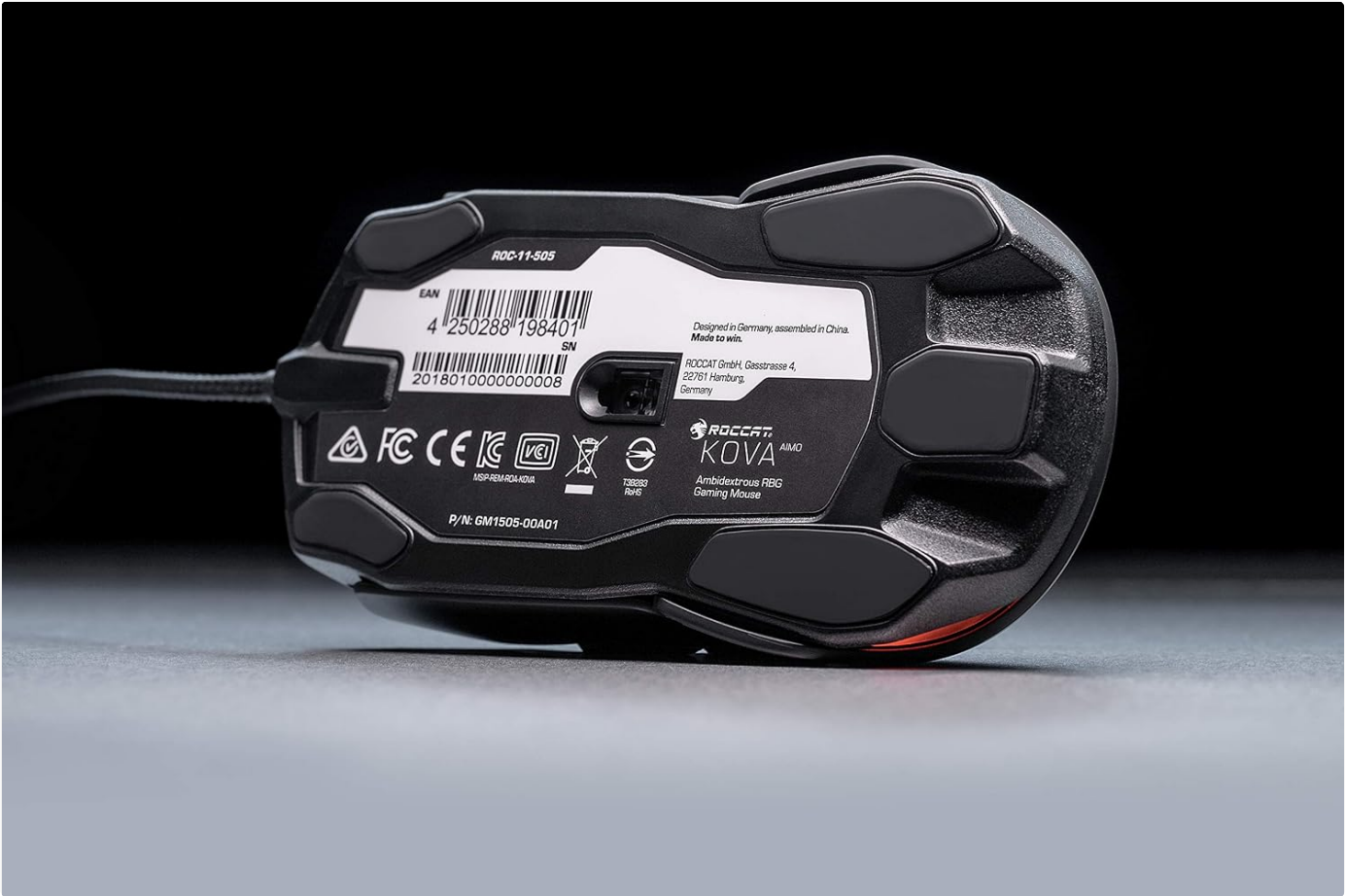
Figure 5: The underside of the ROCCAT Kova AIMO mouse, showing the optical sensor and glide feet.
