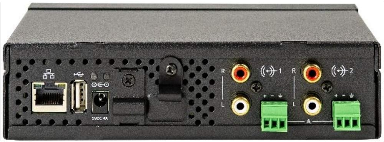
Figure 1: Rear Panel Connections. This image displays the rear panel of the LW-100P-02-01 server, highlighting its connectivity options. From left to right, you can see the Ethernet port (RJ45), a USB Type-A 2.0 port, the 5V DC power input, two sets of RCA audio inputs (Left and Right), and two sets of terminal block connectors for analog audio inputs.
