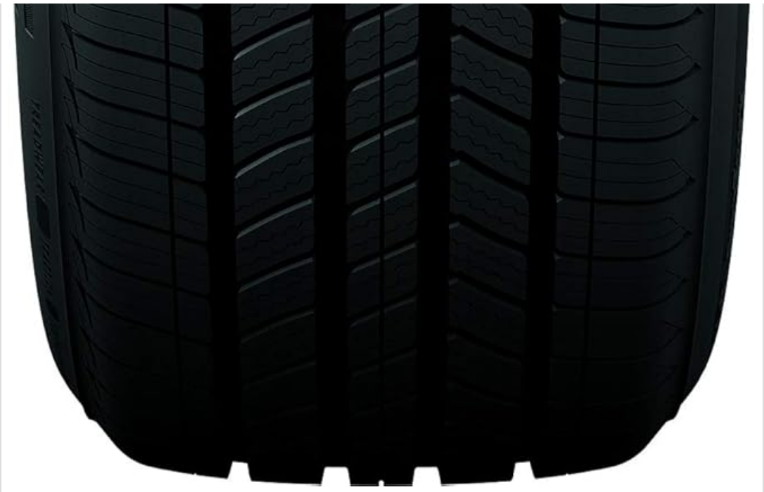
Image: A detailed view of the asymmetrical tread pattern of the Bridgestone Turanza QuietTrack tire, highlighting the sipes and grooves.
