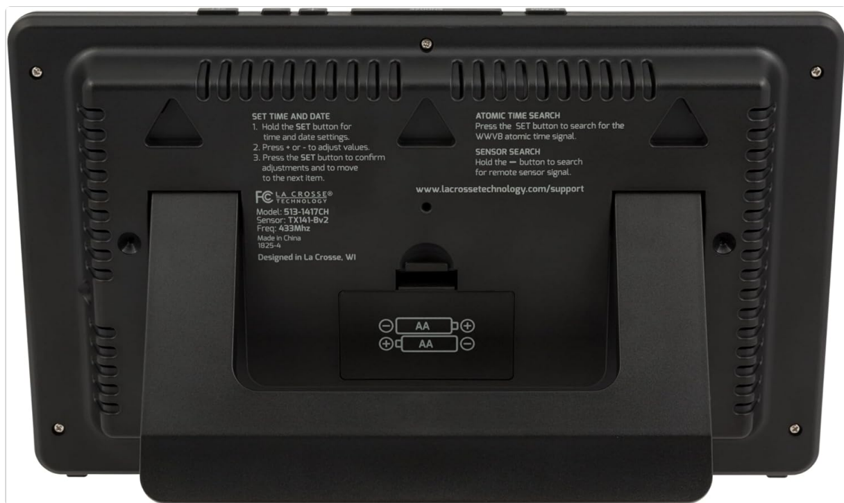
Image: Rear view of the La Crosse Technology Digital Clock, highlighting the battery compartment and printed instructions for setting time, date, atomic time search, and sensor search.
