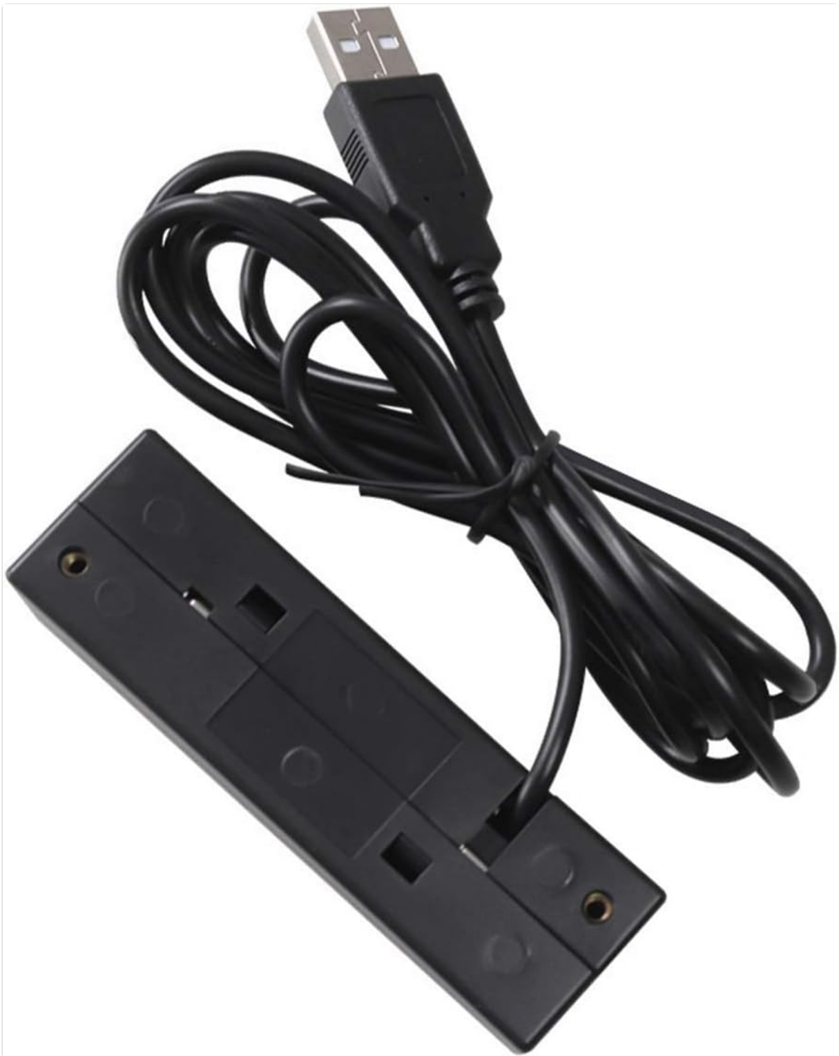
Figure 4: Bottom view of the MSR580 reader, showing mounting points.
