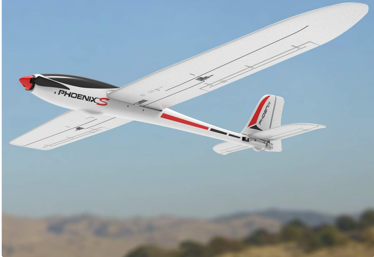
Image 5.2: Folding propellers reduce drag during gliding, increasing flight time.
