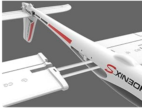
Image 4.2: The Plug & Click Easy Mounting System simplifies wing attachment.
