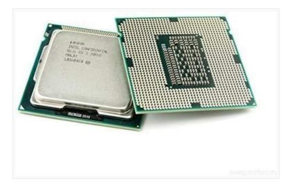
Image: Intel Core i5-3570 processor, displaying the top surface with 'Intel Confidential' markings and the pin-side of another unit, highlighting the LGA 1155 contact points.
