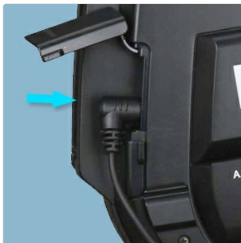
Figure 4: Connecting the remote cord to the camcorder's LANC terminal.
