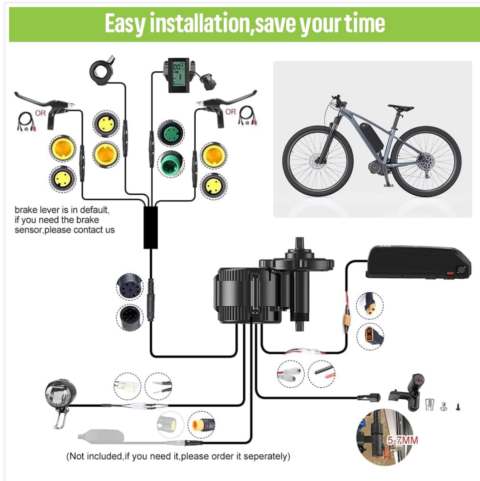
Image 3.2.1: Simplified wiring diagram illustrating connections between the motor, display, throttle, brake sensors, and battery. Note: Brake lever is default; contact seller for brake sensor if needed.
